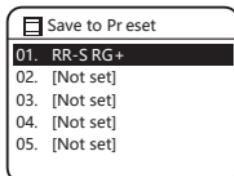
2. Select one of the 30 presets to store the current station by pressing **▶||▲ / ▼** buttons to select the number and press the **SELECT** button to confirm. The display will show “**Preset stored**” and then save the station
